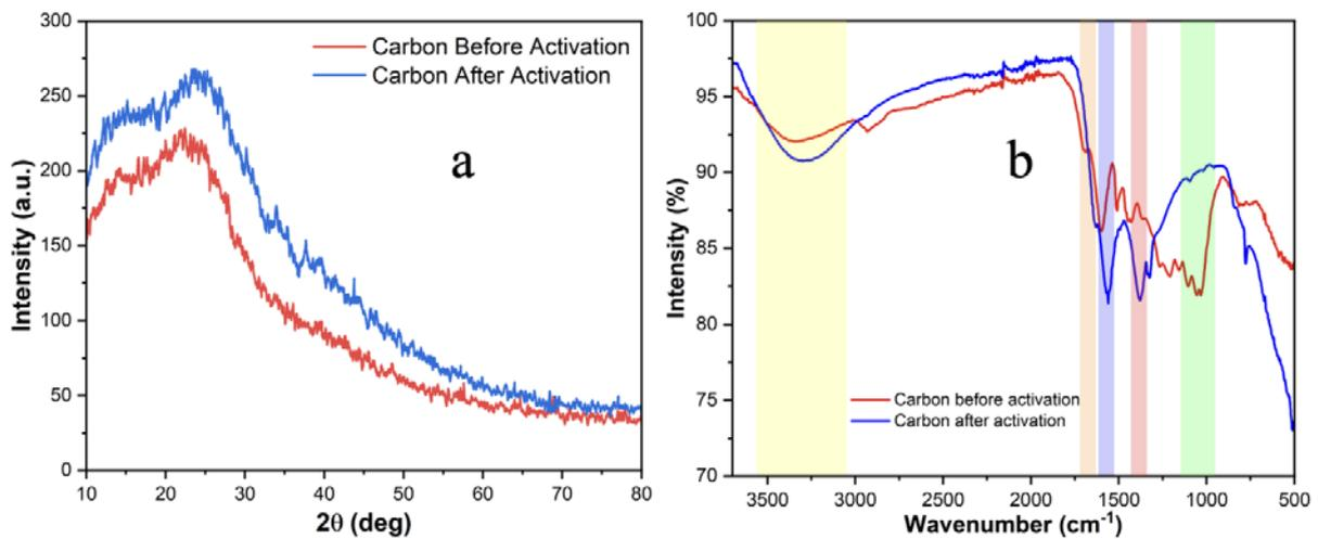
**Figure 2.** (a) XRD diffraction patterns of carbon before and after activation; (b) FTIR spectra of carbon before and after activation.
