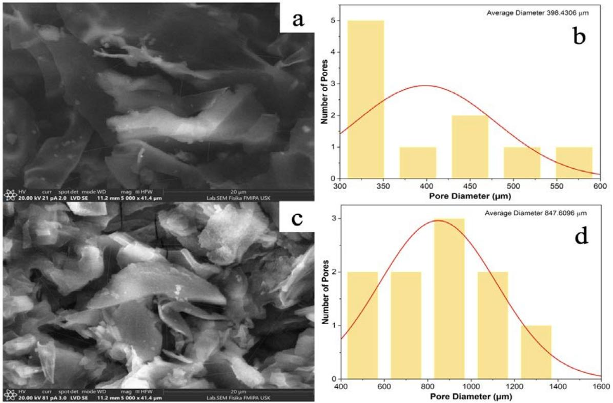
**Figure 1.** SEM images and pore size distribution of activated carbon: (a) morphology before activation, (b) pore size distribution before activation, (c) morphology after activation, (d) pore size distribution after activation.
