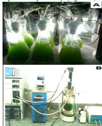
Figure 1. Growth optimization of C. subellipsoidea microalgae in BBM media supplemented with 20%, 40%, 60%, 80% and 100 of sterile/unsterile Dairy using shake flask methods (A) and bioreactor for large scale biomass production & lipid productivity (B).
