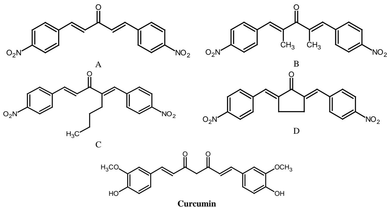
**Figure 1.** 2D Chemical structures of synthesized compounds and curcumin (positive control).
