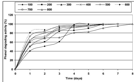
**Figure 7.** Time profiles of phenol biodegradation by immobilized cells of *Bacillus* sp. 2BSG-PDA-16. Error bars represent the standard deviation
