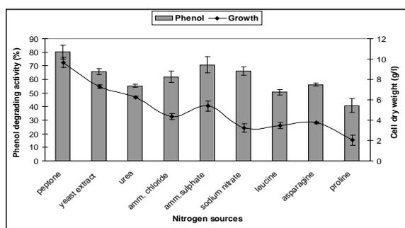
**Figure 3.** Effect of nitrogen sources on growth and phenol degrading activity of *Bacillus* sp. 2BSG-PDA-16. Results are means of three independent determinations and error bars represent the standard deviation
