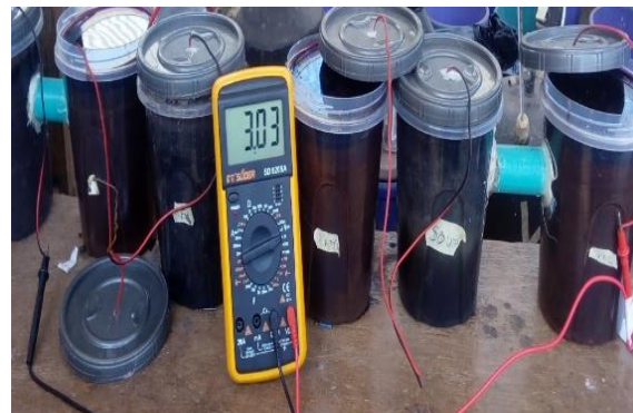
Figure 9: Pig dung based MFCs connected in series generated voltage of 3003 mV
