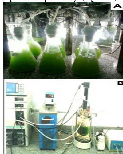
Figure 1. Growth optimization of C. subellipsoidea microalgae in BBM media supplemented with 20%, 40%, 60%, 80% and 100 of sterile/unsterile Dairy using shake flak methods(A) and bioreactor for large scale biomass production & lipid productivity (B).
