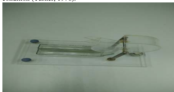
Figure 3. The Folsom plankton splitter used to divide the sample into two halves
