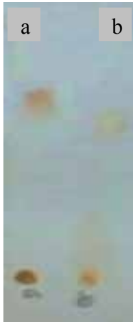
Figure 1. TLC of rutin extract after treatment with ammonium hydroxide ( \text{NH}_4\text{OH} ) solution. a-Standard rutin b- Mature fruit
